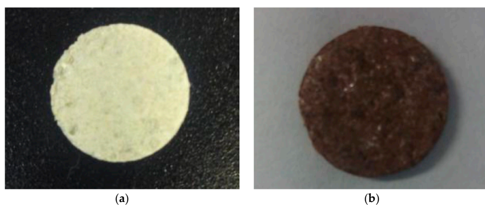
Figure 1. Example of discs made from powder mix for contract angle measure. (a) mica mixed with kaolinite; and (b) mica mixed with kaolinite and aged in crude oil.
