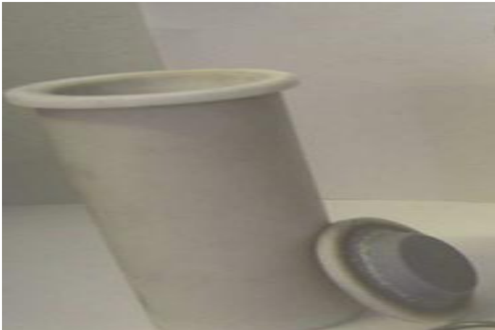
Figure 2.9: The Teflon-lined stainless steel autoclave used in this work
