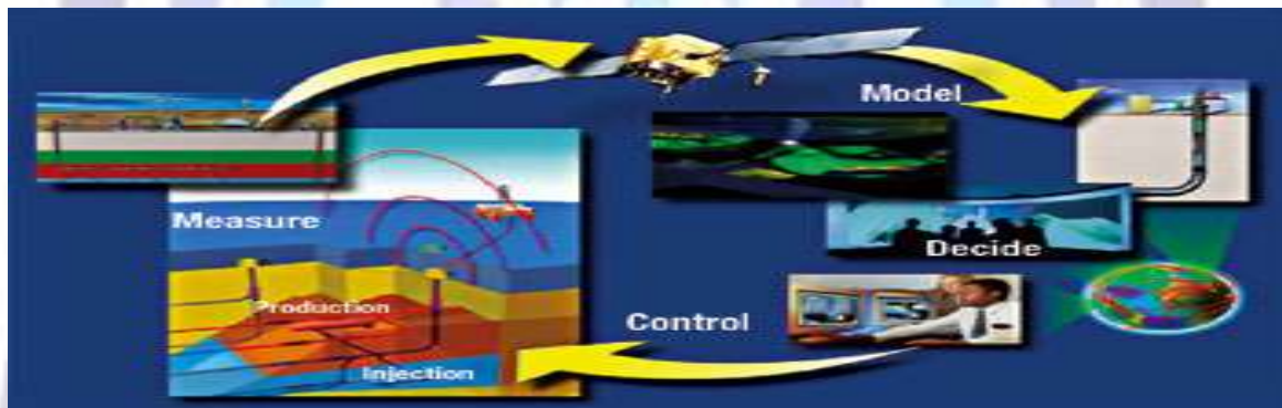
Fig. 2: Shell’s Smart Field Philosophy (measure-model-decide-control loop) [7]
