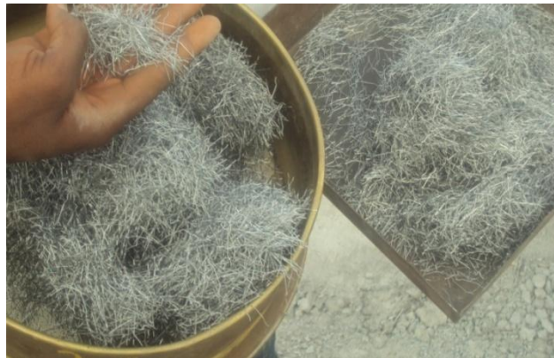
Figure 1. Steel Fibres used (Hooked-end type) [23]
