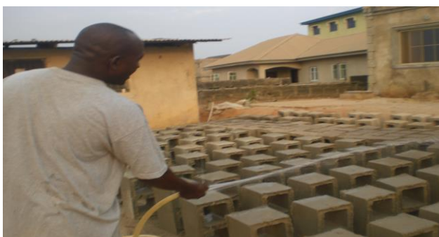
Figure 7: Wetting of blocks at curing section.
