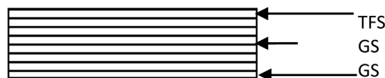
FIG. 4. Composition of the sides of the solar cooker facing the sun and the top.
