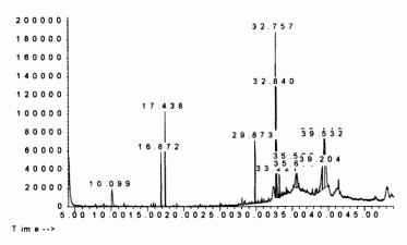
Figure 8: Image of GC-MS analysis on unbleached oil
