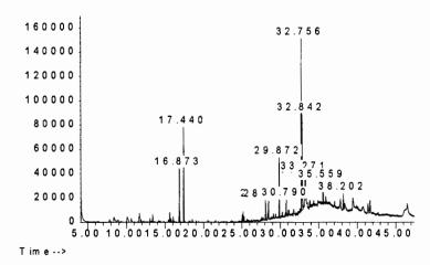
Figure 9: Image of GC-MS analysis on bleached oil
