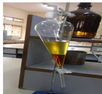
Fig. 1. Layers of Biodiesel (top) and Glycerol
