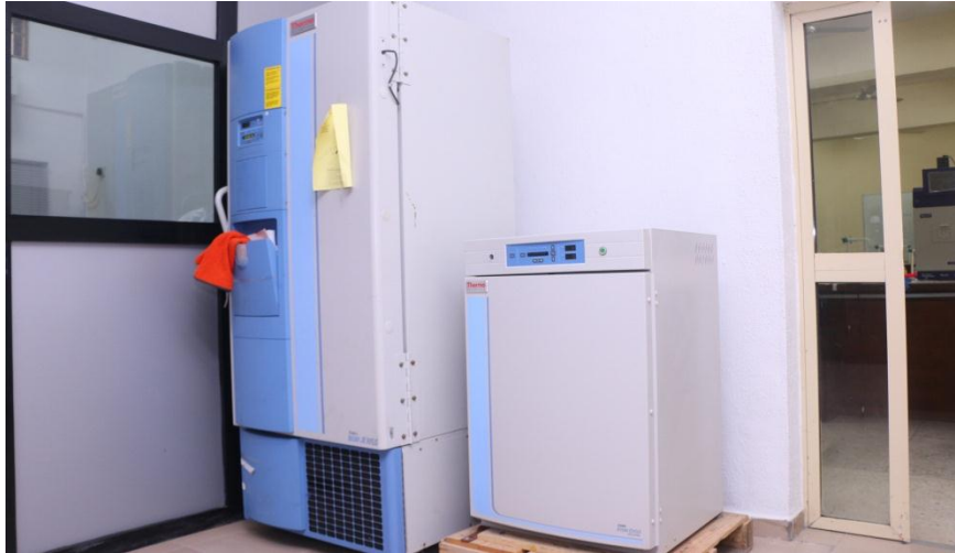
86°C Celcius Ultra Low Temperature Freezer and CO 2 Incubator in the Biological Science Department
