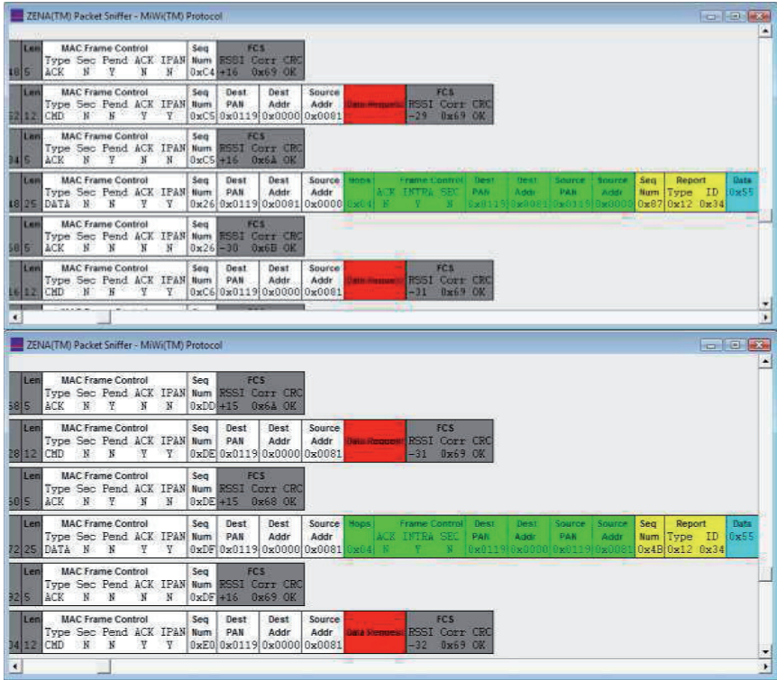
Appendix Figure 5: Transmitted packets between MiWi PAN Coordinator and MiWi End Device
