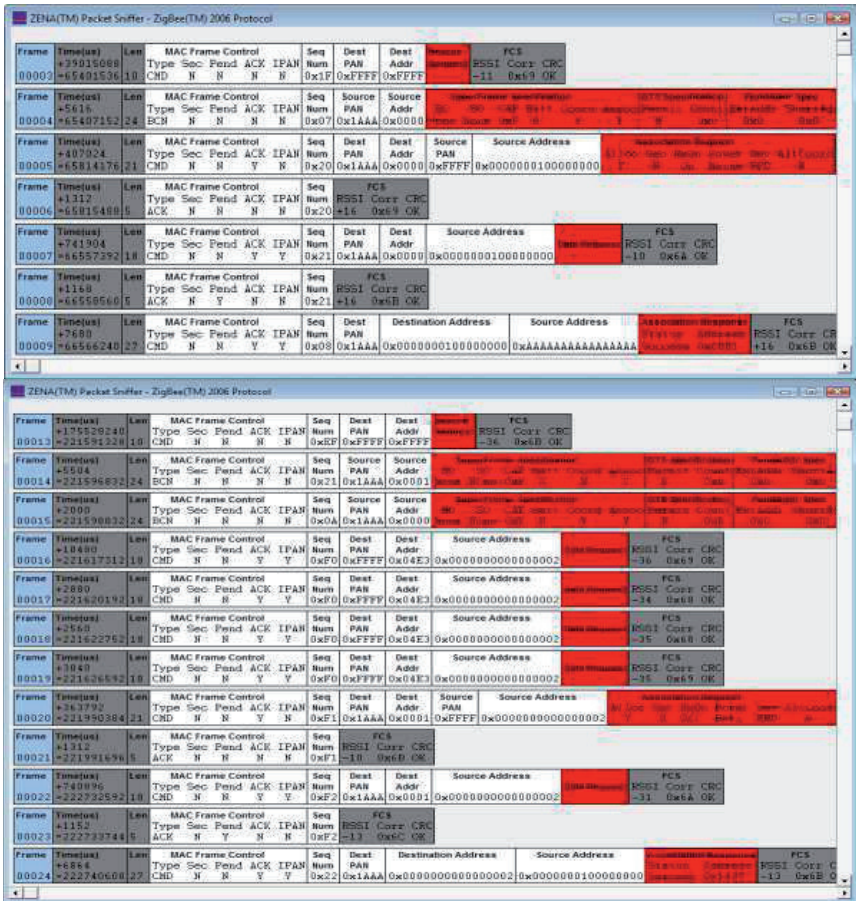
Figure 10: ZENA display of request and response packets between Coordinator, Router and End Device
