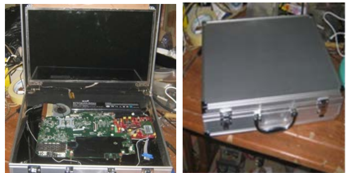
Fig. 6. Assembling of Nomadic Monitoring Unit
