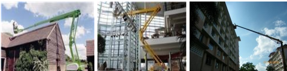
Figure 8 a,b&c: Access work platform
