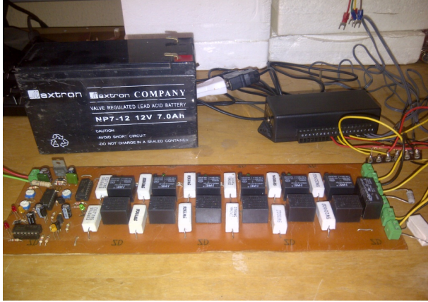
Fig. 5. Photo of the I-V curve tracer
