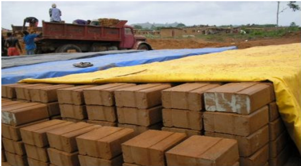
Figure 1: Interlocking blocks, an indigenous material produced from laterite and used in Obasanjo low-cost housing estate, Ado-Ekiti, Nigeria.
