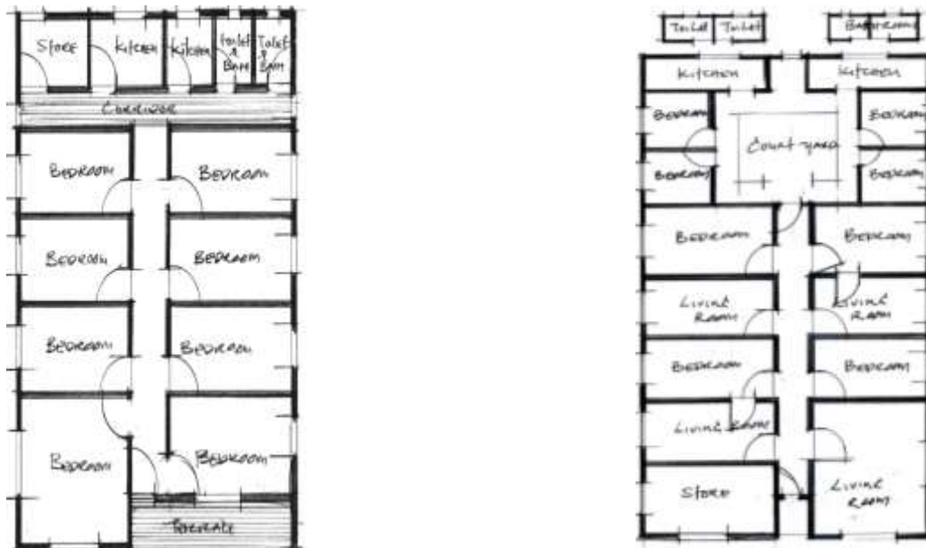
Fig1a & b: A Typical Floor Plan of a Central Corridor House (“Face Me I Face You”)
