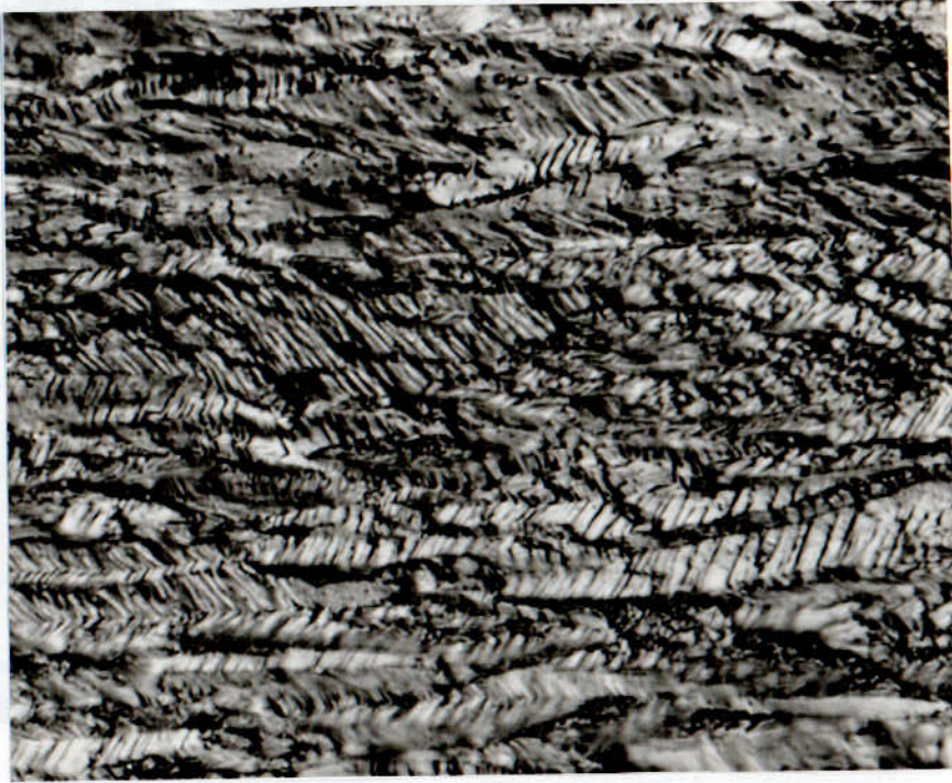
Figure 5.11 Optical microstructure of cold worked nickel subjected to identical regimes of temperature as those used in permeation experiments, annealing time: 24 hrs at 398 K +24 hr at 423 K+ 16 hrs at 448 K, magnification: \times 600
