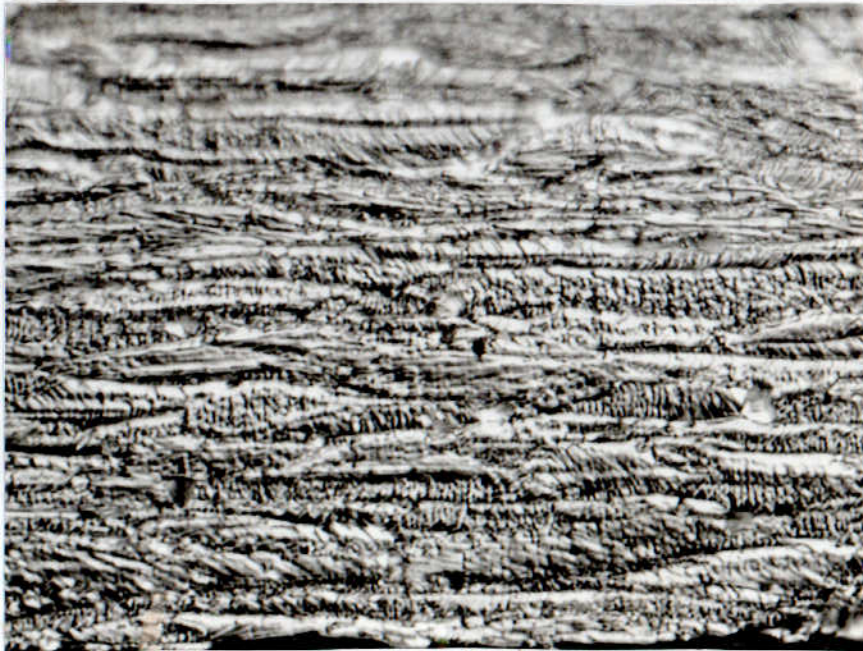
Figure 5.10 Optical microstructure of 87% cold worked nickel, no anneal, magnification: \times 600
