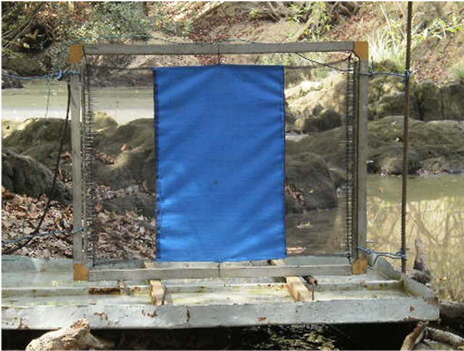
Figure 1. Example of a target design used for comparison. A 0.75 m wide \times 0.50 m high net-blue-net target (37.5 cm \times 50 cm blue surrounded by 2 pieces of net of 18.75 cm \times 50 cm each) inside an electric grid mounted on a fly collection tray. doi:10.1371/journal.pntd.0001332.g001
