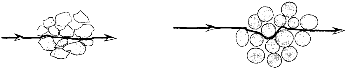
Figure 4-32. Effect of grain sphericity on porosity. (a) Angular grains will produce a greater porosity leading to greater conduction through the sediment. (b) Spherical sediment grains will reduce porosity and conduction.
