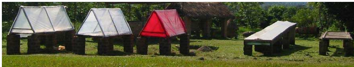
Figure 4-1: Solar dryers. From left to right: UV-polythene resistant; non-UV resistant; red-polythene; tunnel dryer and open sun-air dryer
