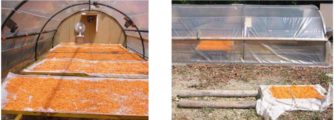
Figure 3-3: Greenhouse solar dryer. Views from the front (left) and the side that includes sun dryer (right).
