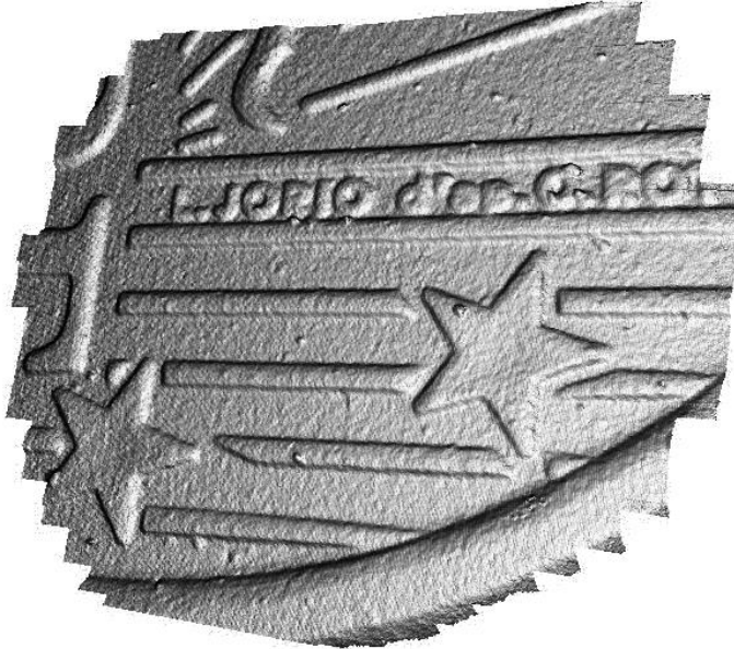
Figure 7 – 3D surface reconstruction of the white painted 10 cents euro coin and with a white light source
