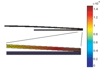
Fig. 1. Deformation of the beam in contact with the substrat
