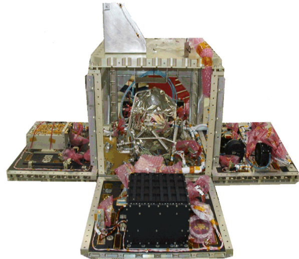
Fig. 9 MYRIADE platform example with the PICARD microsatellite.
