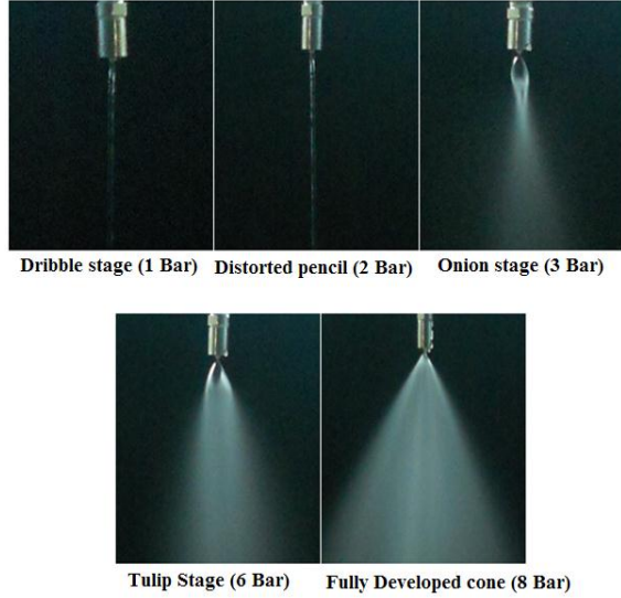
Figure 8: FIVE DIFFERENT STAGES OF SPRAY WITH INCREASE IN INJECTION PRESSURE.
