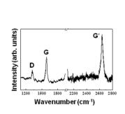
Figure 2. Raman spectrum of as-grown graphene on Cu foils.
