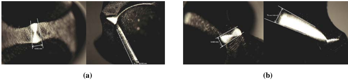
Fig. 2: Typical tool wear pattern for (a) Ni-B coated HSS 5 mm drill bit (b) uncoated HSS 5 mm drill bit, after drilling 100 holes in carbon epoxy laminate.
