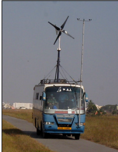
Figure 6(a) Tow Testing at HAL Airstrip, Bengaluru
