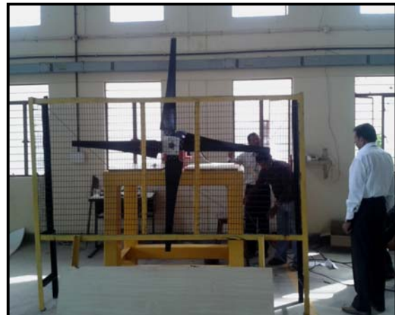
Figure 5(b) Rotor undergoing Spin Test
