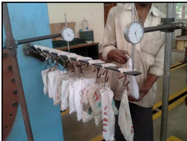
Figure 5(a) Blade under static deflection test
