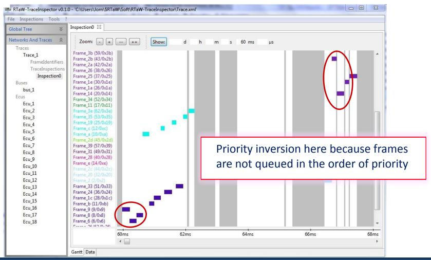
Check comm. stack implementation, periods, offsets, jitters, model for aperiodic traffic and transmission errors, clock drifts, etc .. [*RTaW-Trace Inspector* screenshot]
