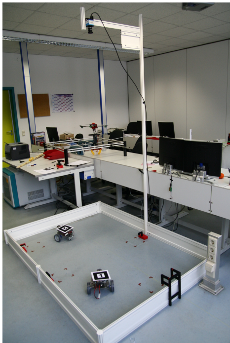
Fig. 2 The experimental testbed with global positioning system.
