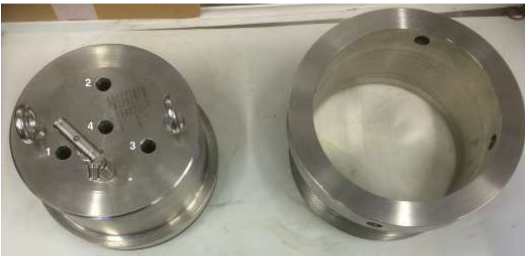
Fig. 3.6 The lid of the IPOCAMP comprises two circular parts. Windows 1, 2, 3 are used to provide lighting; window 4 is used to view the inside of the pressure vessel using an endoscope.
