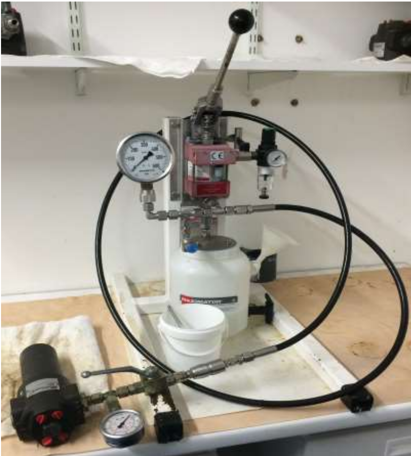
Fig. 3.11 MAXIMATOR hydraulic pump used to pressurize the vessels.
