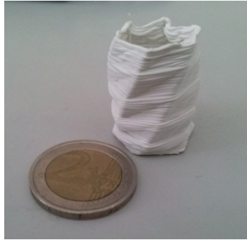
Figure 14 Ceramic vase 3D-printed with composition H0 and heat treated at 1000°C for 1h.
