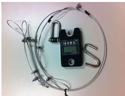
Figure 43: The dynamometer and the steel cable used for conducting the MVC tests.
