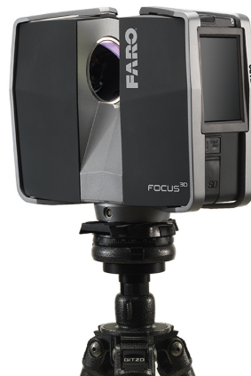
(b) Laser scanner for architecture
