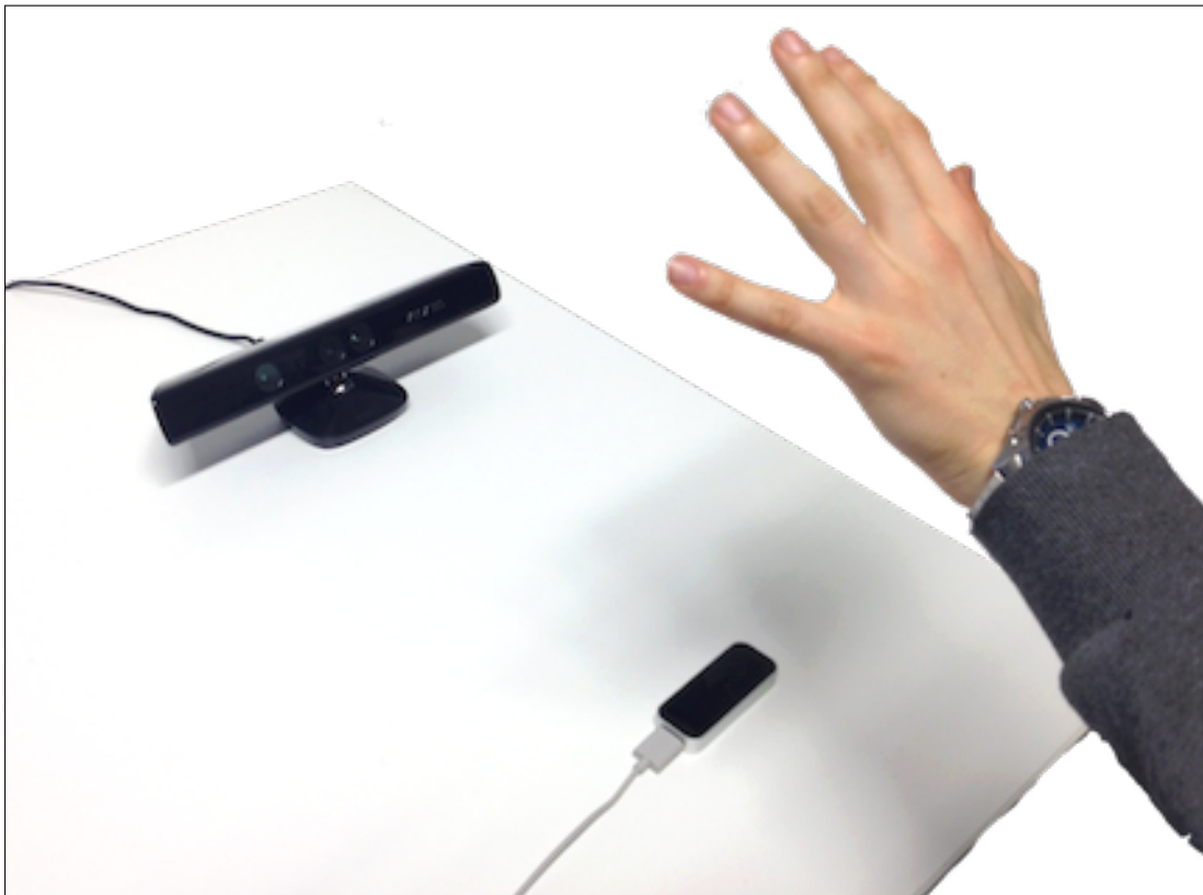
Figure 2.21: Example of hybrid setup made by a Kinect and the Leap Motion
