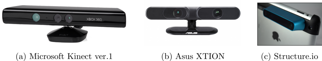
Figure 2.13: Example of available structured light coding low-cost range cameras.
