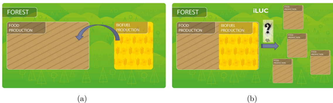
Figure 1.10: Indirect Land Use Change: (a) When Agricultural activity (Food Production) is displaced by crops for biofuel production, there is the need to produce more food somewhere else; (b) that implies that an additional amount of CO 2 emissions are released into the atmosphere (by changing e.g. forest into agricultural land).
