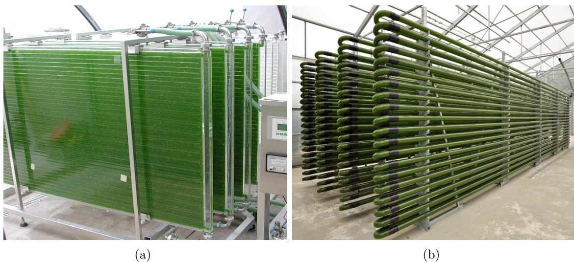
Figure 1.9: Examples of closed photobioreactors as flat plate and tubular reactors.
