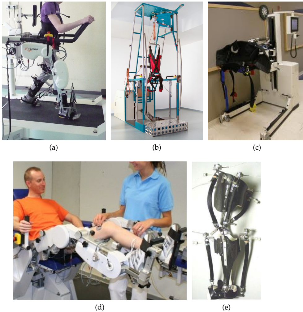
Figure 2: Robotic Assistive Devices for lower limbs rehabilitation: (a) treadmill gait trainers (Lokomat picture courtesy of Hocoma); (b) foot-plate based gait trainers (The Gangtrainer picture courtesy of RehaStim); (c) overground gait trainers (KineAssist picture courtesy of Kinea Design, LLC); (d) stationary gait and ankle trainers (The MotionMaker picture courtesy of Swortec SA), and (e) active foot orthoses (KAFO picture courtesy of Prof. Ferris, University of Michigan).
