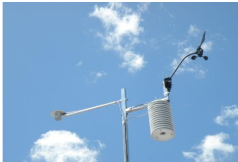
Figure 6.26 Weather station integrating the pyranometer, the air temperature thermometer and the anemometer
