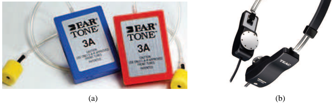
Figure 1.13: Etymotic ER-1 insert headphones ( http://www.etymotic.com/pro/er1.aspx ) and Teac Filltune HP-F100 bone-conduction transducers ( http://teac-ipd.com/ ) (devices used by Stanley (2009) in his studies).
