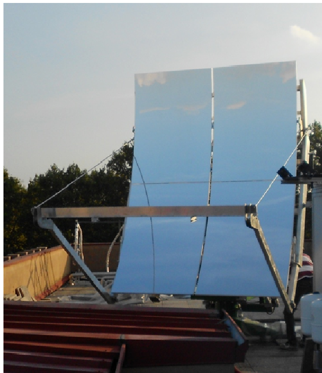
Figure 6.4. Prototype of the semi-parabolic trough linear concentrator installed at the University of Padova.
