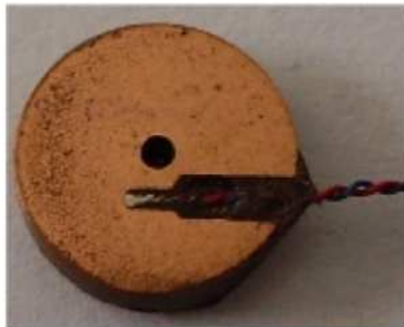
Figure 3.3.4. Enlarged image of the cross section of the fin sample showing the accommodation of a wall thermocouple.
