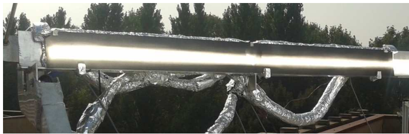
Figure 6.7. Thermal receiver during a test run. The sunlight is concentrated on the absorber with selective coating.
