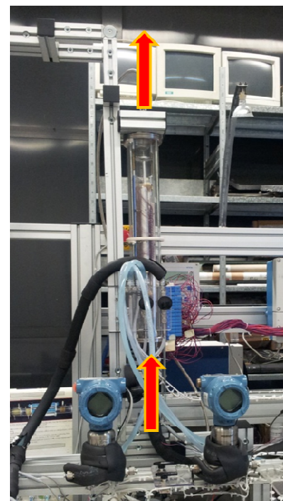
Figure 4.4. Different orientation of the test section to study the effect of inclination in condensation: Left:45° downflow; Right: vertical upflow.
