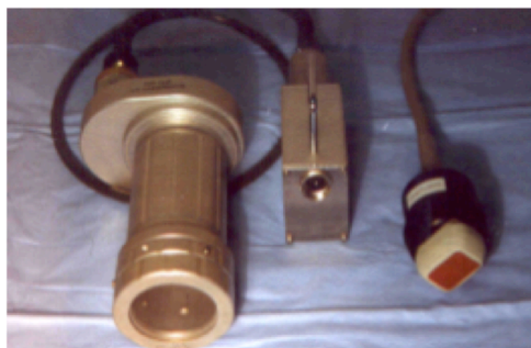
Figure 2.9. Motorized device that housed an external stepper motor that mechanically rotated a built-in transthoracic transducer.
