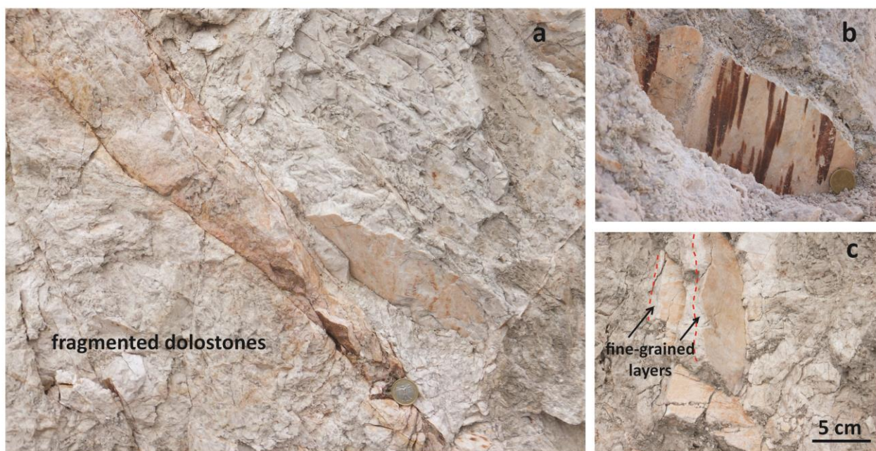
Fig.6 Fault networks cutting fragmented dolostones of the FFZ. (a) Two sub-parallel minor faults with sharp slip surfaces cutting through fragmented dolostones. (b) Detail of a “mirror-like” slip surface containing brownish flames of iron oxide and hydroxides (hematite and goethite from XRPD analyses) elongated along fault striae. (c) Two mirror-like faults cutting through fragmented dolostones. The faults contain up to a few centimeters of fine-grained whitish fault rock.
