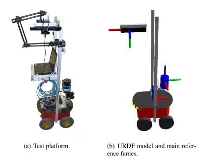
Figure B.6: (a) The robotic platform used in the KTP dataset and (b) its URDF model together with the main reference frames. Note that for this dataset we only acquired RGB-D data from a Microsoft Kinect sensor and did not make use of other sensors such as Laser Range Finder or sonars.
