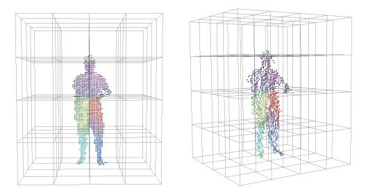
Figure 5.3: Two different views of the computed 3D grid: 4 partitions along the x, y and z axis are used.
