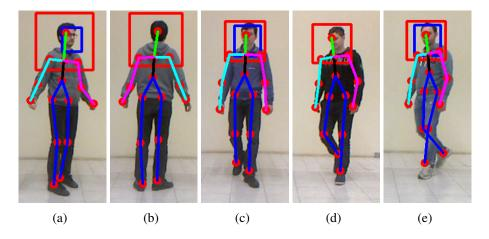
Figure A.4: Example of skeleton estimation obtained with NiTE skeletal tracker and face detection guided by the skeleton tracking.
