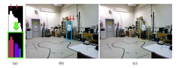
Figure 3.8: Example of how the sub-clustering method allows to correctly detect a person otherwise merged with the background. a) Height maps, b) detector output, c) tracker output.
