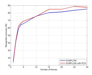
Figure 5.8: Mean recognition accuracy when varying the number of frames used for composing the sequence descriptor.
