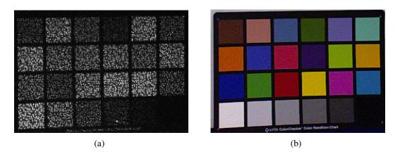
Figure 2.13: (a) Reflection of Kinect infrared pattern when projected on the color palette in (b). Figure courtesy of [29].
