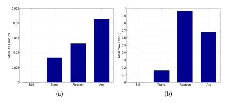
Figure B.7: Histograms of the odometry error ((a) in *x*-*y* and (b) in *yaw*) with respect to the ground truth obtained with the marker-based motion capture system.
