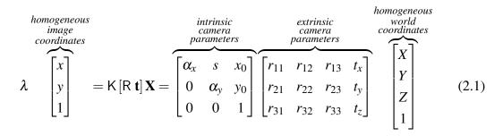
where K is the matrix containing the intrinsic parameters of the camera (focal lengths, optical center and skew), while R and t contain the rotation and translation parameters from world to camera reference frame [92].
