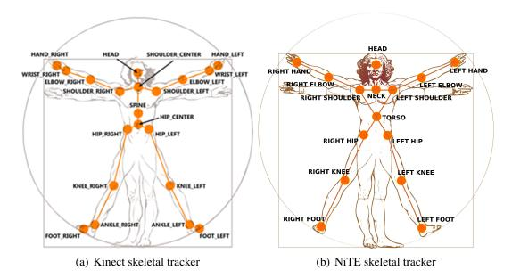
Figure A.1: Position and names of the human skeleton joints estimated with (a) Kinect skeletal tracker and (b) NiTE skeletal tracker.
