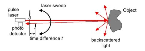
Figure 2.7: Illustration of a 2D laser range finder with rotating mirror based on the laser pulse time-of-flight principle. Figure courtesy of [50].
