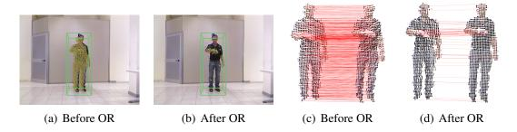
Figure 5.2: Example of 3D flow estimation results reprojected to the image (a-b) for action *Check watch*. Flow is visualized as green arrows in the image, (a) before and (b) after outlier removal (OR). Also correspondences between point clouds are visualized (c) without and (d) with outlier removal.
