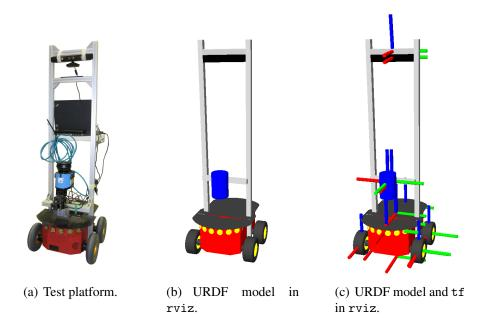
Figure 3.14: The robotic platform (a) used in the tests, its model displayed with the ROS visualizer (b) and the reference frames of every model joint (c).
