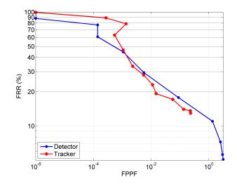
Figure 3.7: DET curve comparing the detector and tracker performance on the KTP dataset in terms of False Positives Per Frame (FPPF) and False Rejection Rate (FRR).
