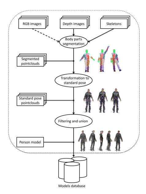
Figure 4.10: Illustration of the pipeline we developed for creating full 3D models of freely moving persons. RGB information is added to the point cloud models only for a better visualization, but in this work it is not used for matching.
