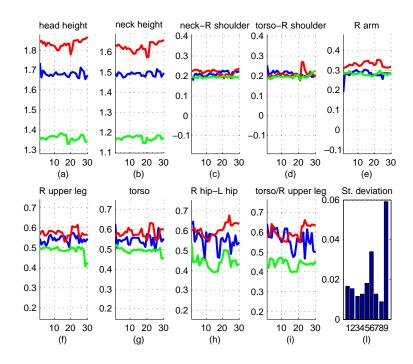
Figure 4.15: (a-i) Estimated skeleton features for some frames of the *Walking* test sequence for the three subjects of Figure 4.13. Those subjects are represented by blue, red and green curves, respectively. In (l), the standard deviation of these features is reported.
