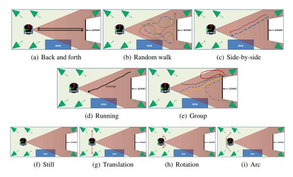
Figure B.4: Illustration of (a-e) the five situations featured in the KTP dataset and (fi) the four movements the robot performed inside the motion capture room. Motion capture cameras are drawn as green triangles, while Kinect field of view is represented as a red cone.
