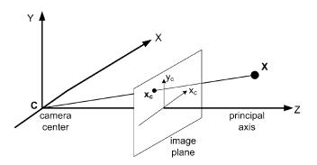
Figure 2.1: Perspective projection based on the pinhole camera model. Figure courtesy of [92].
