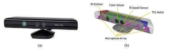
Figure 2.11: (a) External view of the Microsoft Kinect sensor and (b) description of its internal components.
