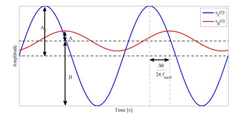
Figure 2.9: Example of emitted signal  $s_E(t)$  (in blue) and received signal  $s_R(t)$  (in red). Figure courtesy of [29].
