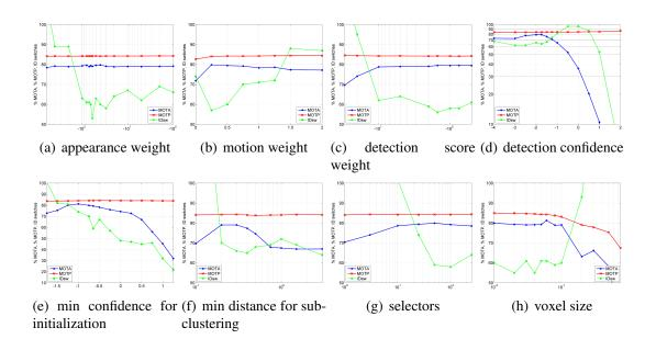
Figure 3.18: Performance of our algorithm on the KTP dataset when varying its main parameters. MOTA (blue) and MOTP (red) curves represent percentages, while ID switches (green) is the number obtained by summing up the ID switches for every video of the dataset. The optimum is reached when MOTA and MOTP are maximum and ID switches are minimum. In some of them, the logarithmic scale is used for the x or y axis for better visualization. Please, see text for details.
