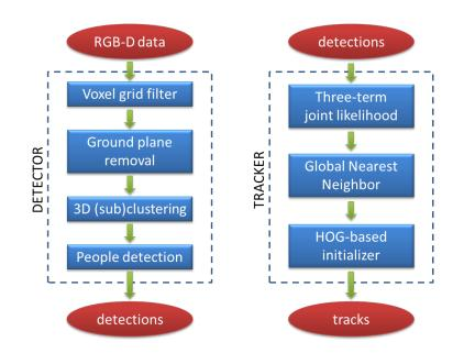
Figure 3.2: Block diagram describing input/output data and the main operations performed by our detection and tracking modules.
