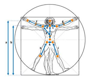
Figure 4.12: Illustration of the links lengths and joints distances to the ground which constitute the skeleton descriptor.
