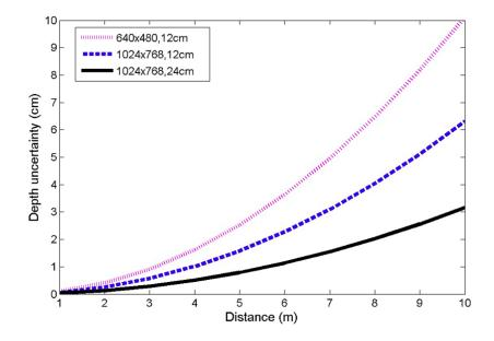
Figure 2.3: Plot illustrating depth estimation uncertainty with respect to distance from the sensor for three different stereo configurations. Figure courtesy of [92].
