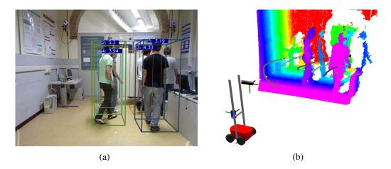
Figure 3.1: Example of our system output: (a) a 3D bounding box is drawn for every tracked person on the RGB image, (b) the corresponding 3D point cloud is reported, together with the estimated people trajectories.
