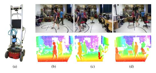
Figure B.1: (a) The platform we used for collecting the IAS-Lab People Tracking dataset and (b-d) some sample RGB images and corresponding 3D point clouds from the dataset.
