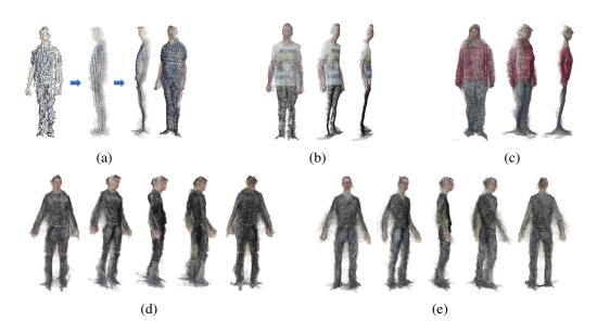
Figure 4.11: (a) Steps of model creation (from left to right: a single person's point cloud, the union of point clouds before and after smoothing); (b-c) examples of  $180^{\circ}$  person models obtained with Kinect skeletal tracker; (d-e) examples of  $360^{\circ}$  person models obtained with NiTE skeletal tracker.
