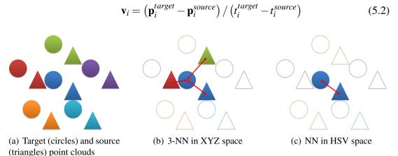
Figure 5.1: Illustration of the matching process between points of two point clouds represented by circles and triangles, respectively. In particular, a point of the target point cloud (blue circle) is matched with the corresponding point of the source point cloud (blue triangle) after (b) K-Nearest Neighbor (K-NN) in XYZ space with K=3 and (c) Nearest Neighbor (NN) in HSV space among the points obtained at the K-NN
