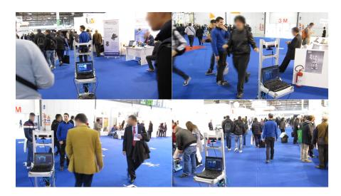
Figure 3.27: Sample images of our mobile robot following the person with the blue sweater within a crowded environment. It is worth noting that the sweater has the same color of the carpet on the floor, thus algorithms based only on color information would have easily failed.
