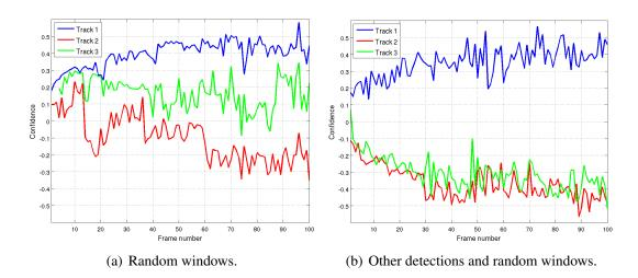
Figure 3.11: Confidence obtained by applying to the three people of Figure 3.10 (b) the color classifier trained on one of them (Track 1) for two different methods of choosing the negative examples.
