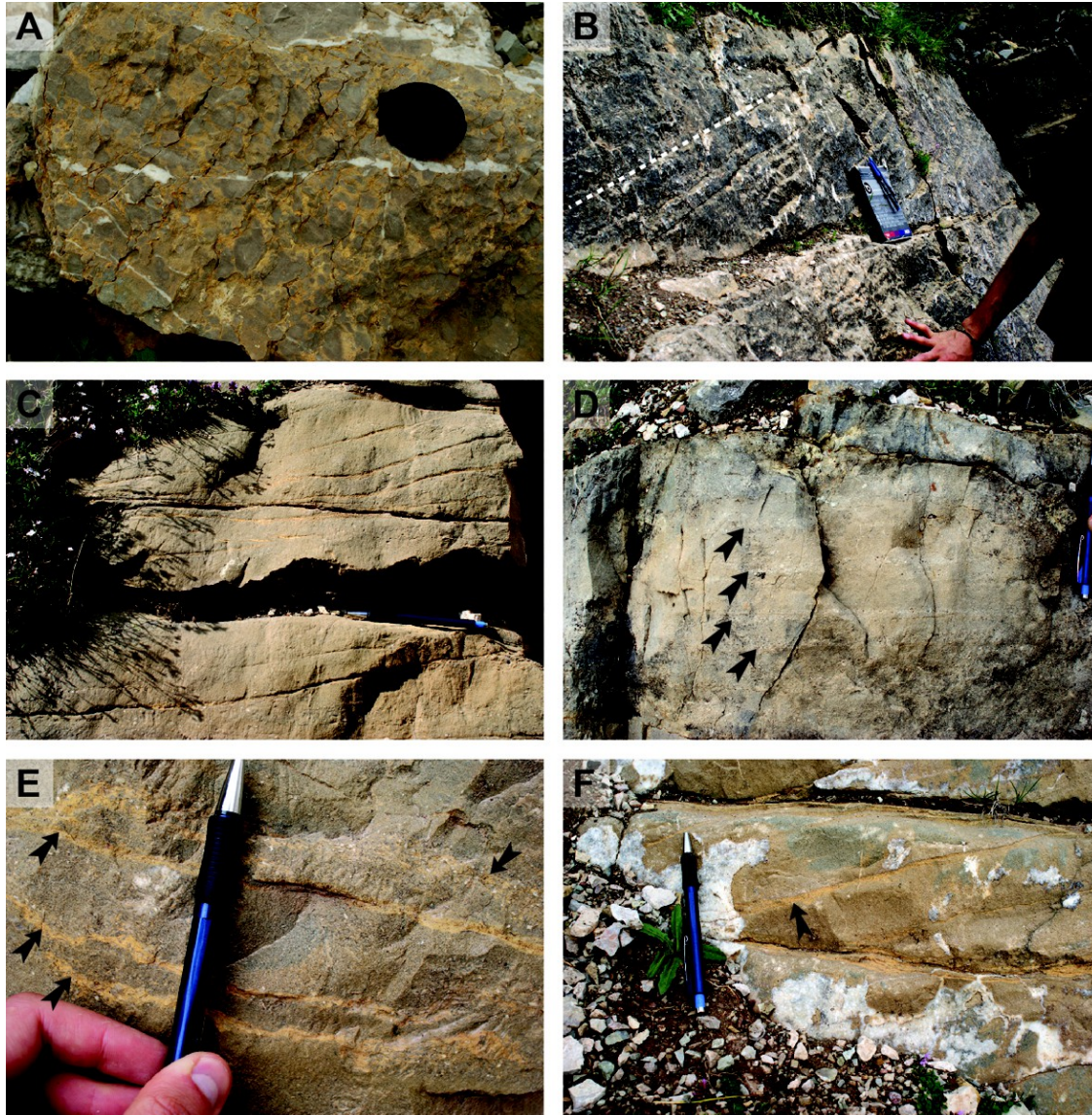
Fig. 3.5. Facies of the Heiligkreuz Fm. observed at Dibona Hut. (A) Flat pebble breccia made up of unconsolidated rip-up clasts (facies L2; interval 2). Both lithoclasts and matrix are constituted of lime-mudstone (B) Calcarenite bed displaying well developed planar cross stratification with an angular basal contact (facies M2; interval 2). White dashed line highlights the stratification. (C) Calcarenite bed displaying well developed planar cross stratification with a tangential basal contact (facies M2; interval 2). Note the yellowish bioclastic-muddy interbeds. (D) Calcarenite bed displaying alternation between mainly oolitic laminae and mainly bioclastic laminae (facies M2; interval 2). Black arrows indicate whitish bioclastic levels. (E) Calcarenite bed displaying alternation between mainly oolitic-siliciclastic laminae and mainly bioclastic-muddy laminae (facies M2; interval 2). Black arrows indicate yellowish bioclastic-muddy levels. (F) Calcarenite bed displaying alternation between mainly oolitic-siliciclastic laminae and mainly muddy laminae (facies M2; interval 2). The black arrow indicates a yellowish muddy lamina which decreases in thickness towards the upper contact.
