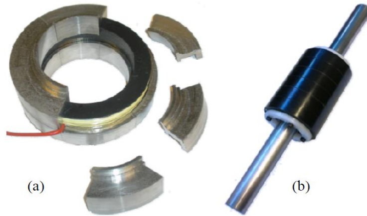
Figure 5.3. TPMLG prototype; (a): stator assembly with twelve SMC modular cores; (b): mover consisting of bonded PM ring mounted on a steel shaft.
