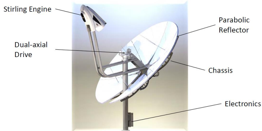
Figure 1.5. Solar dish Stirling cogeneration system.
