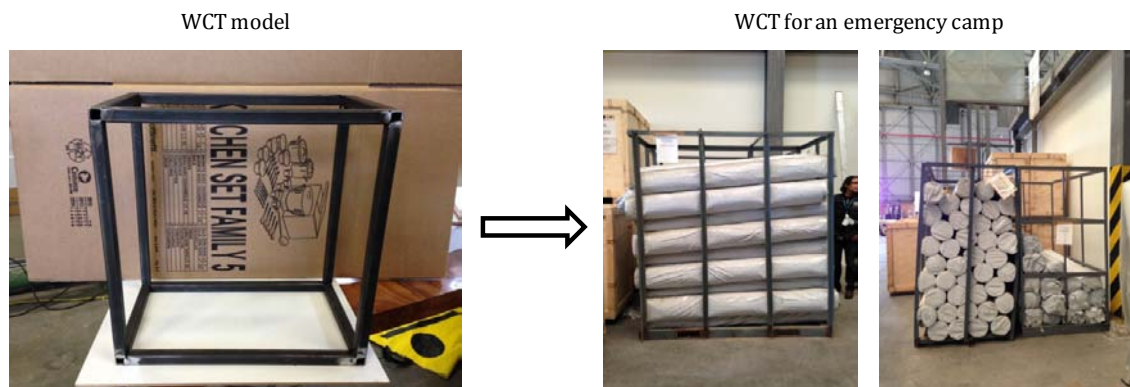
Figure 8.71. The iron cage of the WCT model (on the left) and the steel crate to build the WCT for an emergency camp (on the right)
