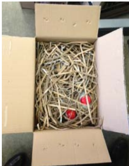
Figure 9.7. Cardboard strips deriving from the cutting of incoming secondary packages used as accessories
