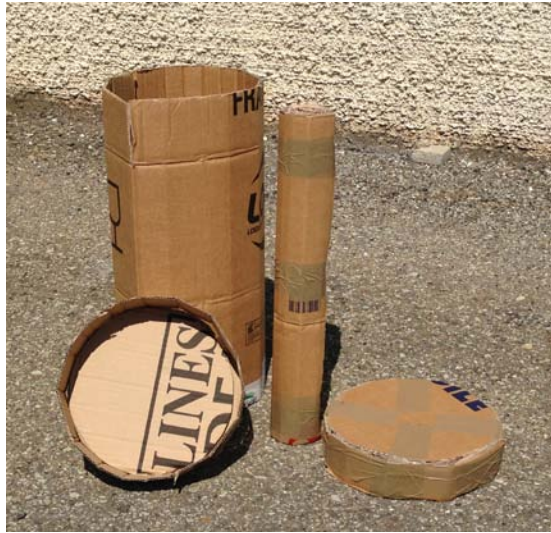
Figure 8.37. The elements composing the carton stool (from the left side: the first cover, the cylinder, the tube and the second cover)
