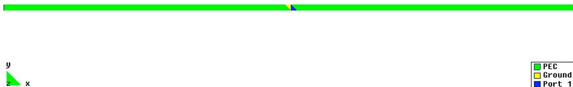
Figure 5.6: Dipole geometry, with length L_d = 3.0 m, and width w = 0.03 m. The dipole is excited in the middle by a voltage gap providing V_0 = 1.0 V.
