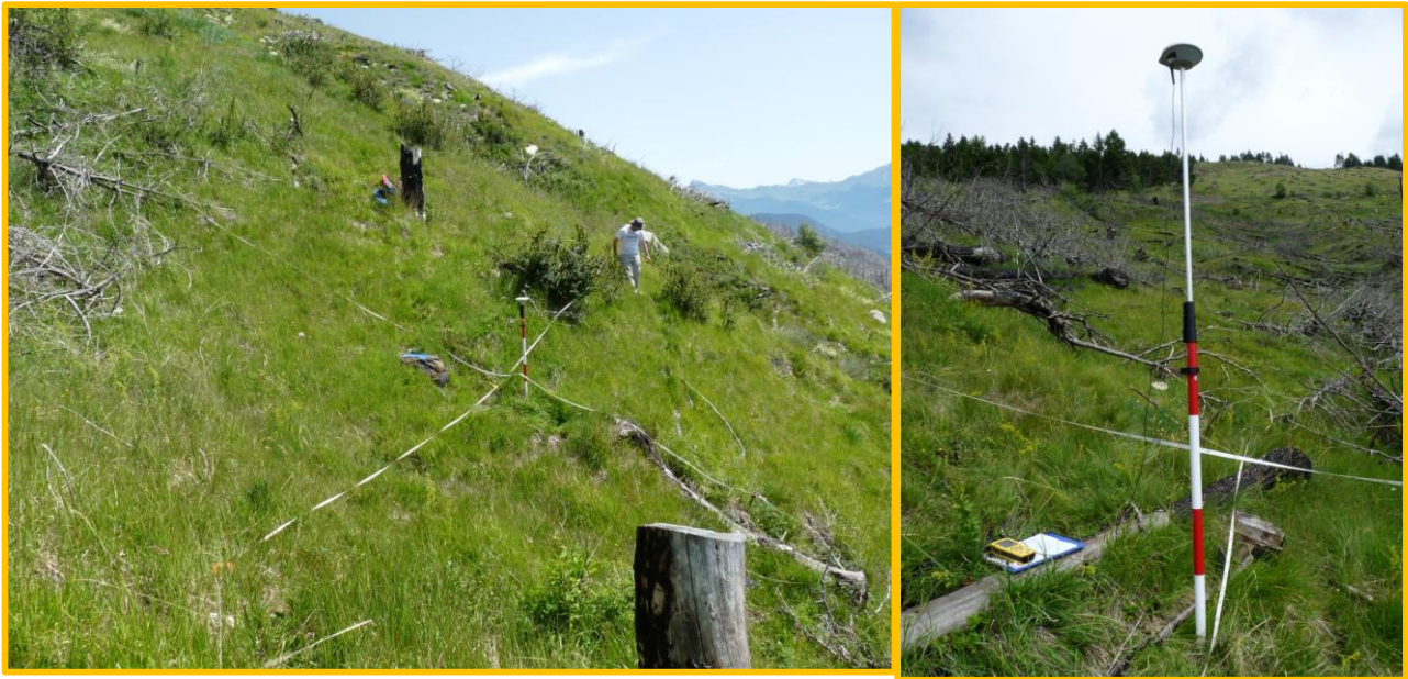
Figure 3.4 -Left: setting up of a sampling plot (circular shape, 6 m radius) within a salvaged area. Right: detailed view of a GPS antenna placed to the plot center.
