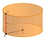
$$V_{cilindro} = A_{base} \times h = \pi \times r^2 \times h = 3.14 \times (30)^2 \times 135 = 3.14 \times 900 \times 135 = 381510 cm^3$$
