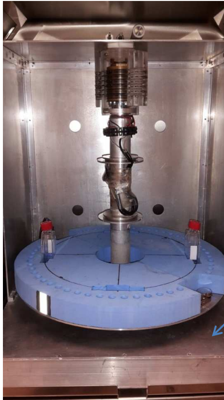
Figure 7: Multi Sample Incubator Centrifuge: for incubation during hypergravity conditions of cell cultures different inserts have been constructed. Depending on the experimental demands, accelerations up to 40 g under controlled environmental conditions can be applied. 1 g controls are located at the side of the centrifuge (arrow) (DLR, Cologne, Germany).
