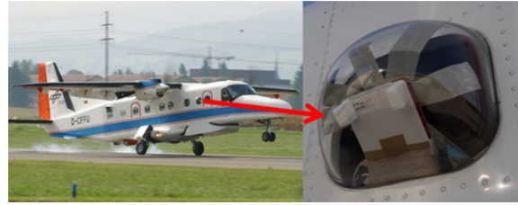
Fig. 2. DLR's DO 228-212 research aircraft (left) and right observation window with provisionally installed LTE FRITZ!Box modem (right).
