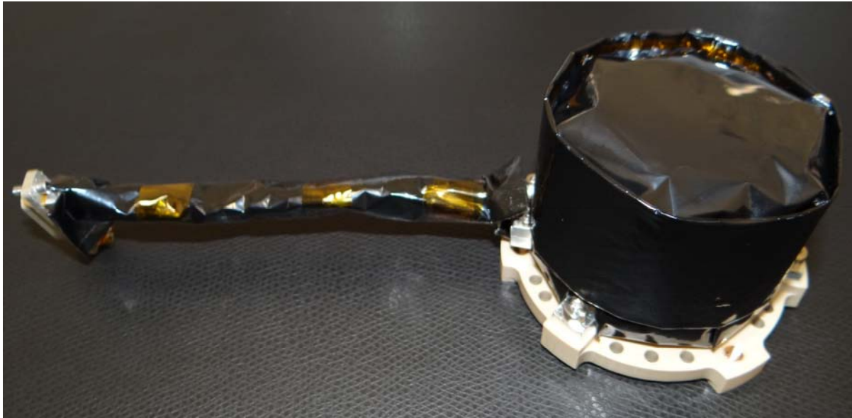
Figure 7 - Magnetometer FM sensor head with a pigtail harness covered with black MLI to eliminate any reflections to MASCOT camera instrument
