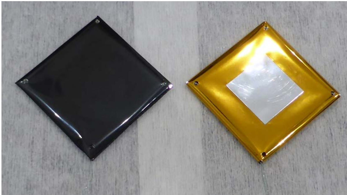
Figure 21: Flight model (FM) of the black (right) and soil (left) type OTS
